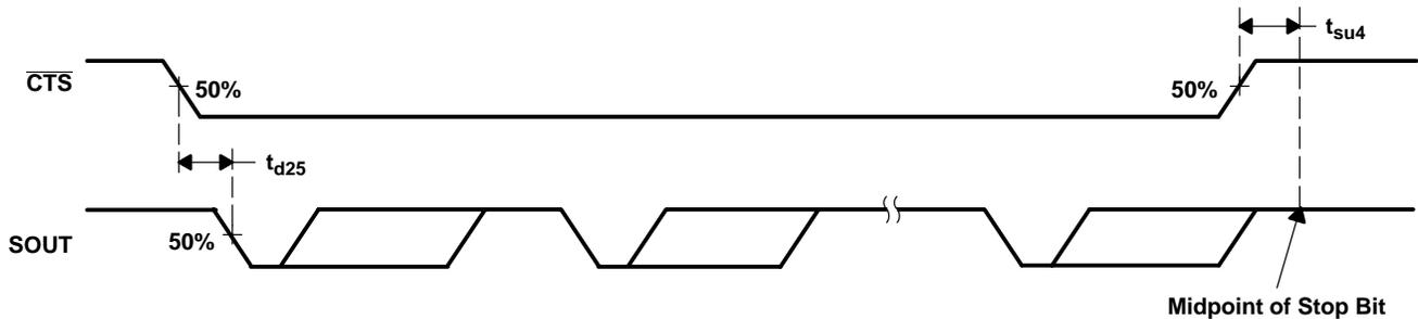
Figure 17.  $\overline{\text{CTS}}$  and  $\text{SOUT}$  Autoflow Control Timing (Start and Stop) Waveforms
