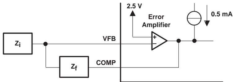
NOTE A: Error amplifier can source or sink up to 0.5 mA.
