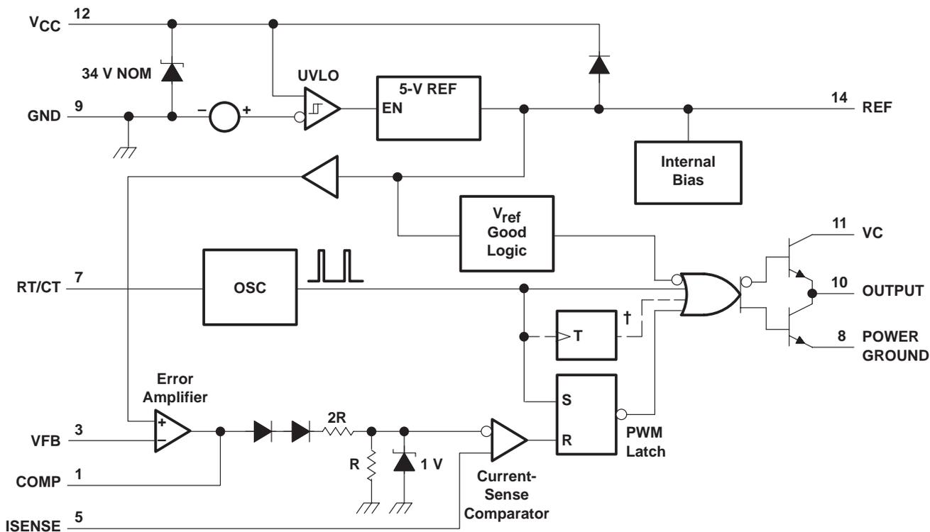
† The toggle flip-flop is present only in TL2844, TL2845, TL3844, and TL3845. Pin numbers shown are for the D Package.
