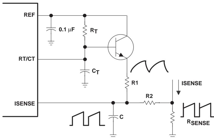
Figure 8. Slope Compensation
