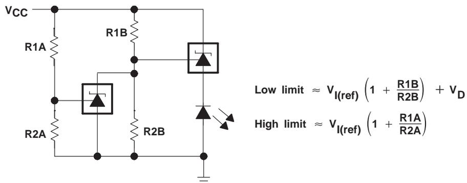
Figure 11. V<sub>CC</sub> Monitor
