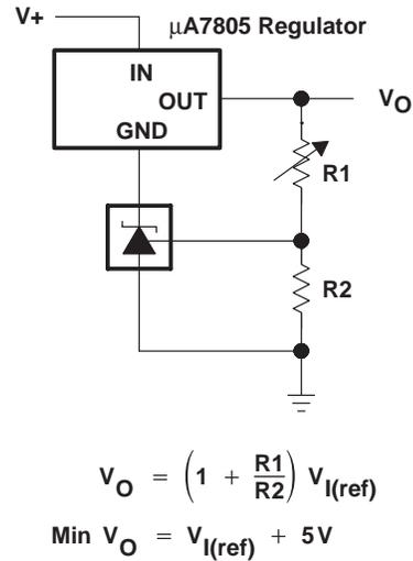
Figure 8. Output Control of a 3-Terminal Fixed Regulator
