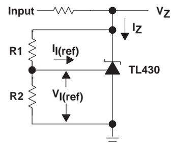
$$V_Z = V_{I(\text{ref})} \left( 1 + \frac{R_1}{R_2} \right) + I_{I(\text{ref})} \times R_1$$
