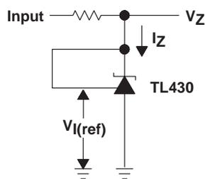
Figure 1. Test Circuit for  $V_Z = V_{I(\text{ref})}$
