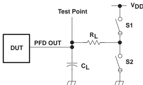
Figure 3. PFD Output Test Condition
