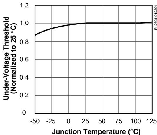
Figure 30. Undervoltage Threshold vs. Temperature.
