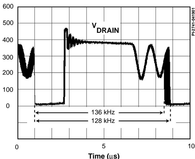
Figure 4. Frequency Jitter.
