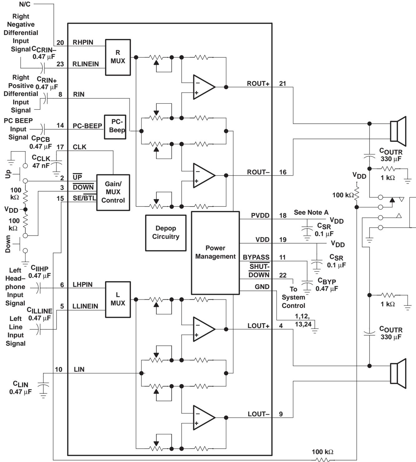
NOTE A: A 0.1 μF ceramic capacitor should be placed as close as possible to the IC. For filtering lower-frequency noise signals, a larger electrolytic capacitor of 10 μF or greater should be placed near the audio power amplifier.
