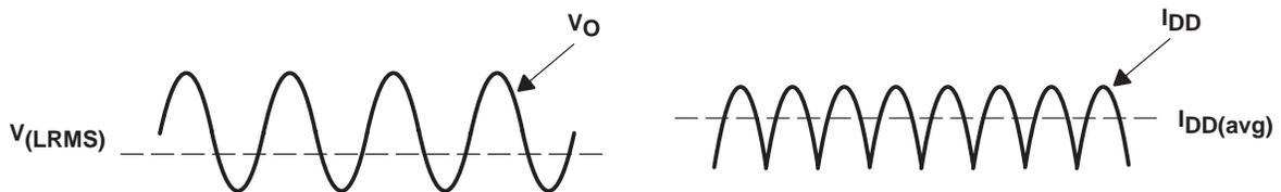
**Figure 34. Voltage and Current Waveforms for BTL Amplifiers**
