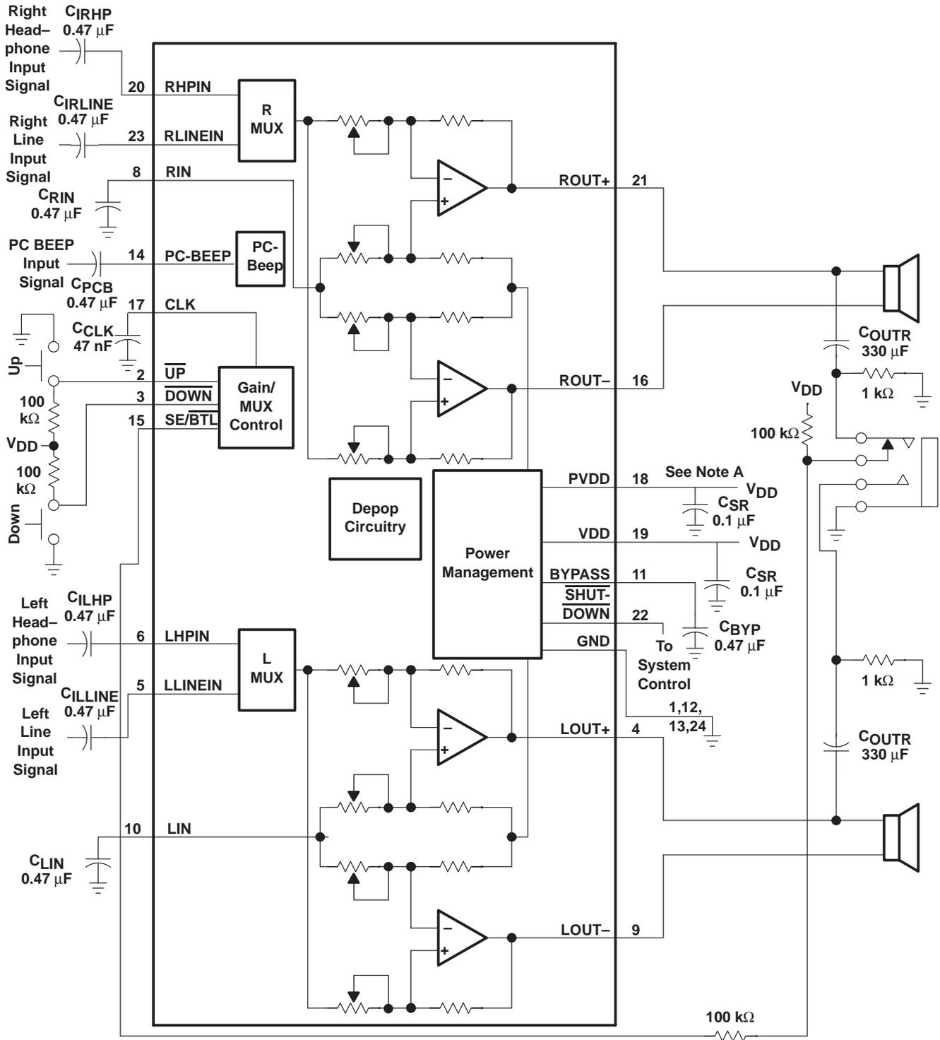
NOTE A: A 0.1 µF ceramic capacitor should be placed as close as possible to the IC. For filtering lower-frequency noise signals, a larger electrolytic capacitor of 10 µF or greater should be placed near the audio power amplifier.
