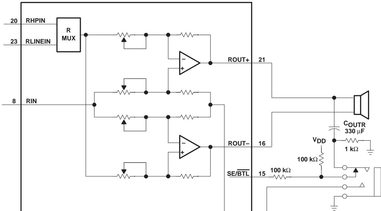
**Figure 35. TPA0162 Resistor Divider Network Circuit**
