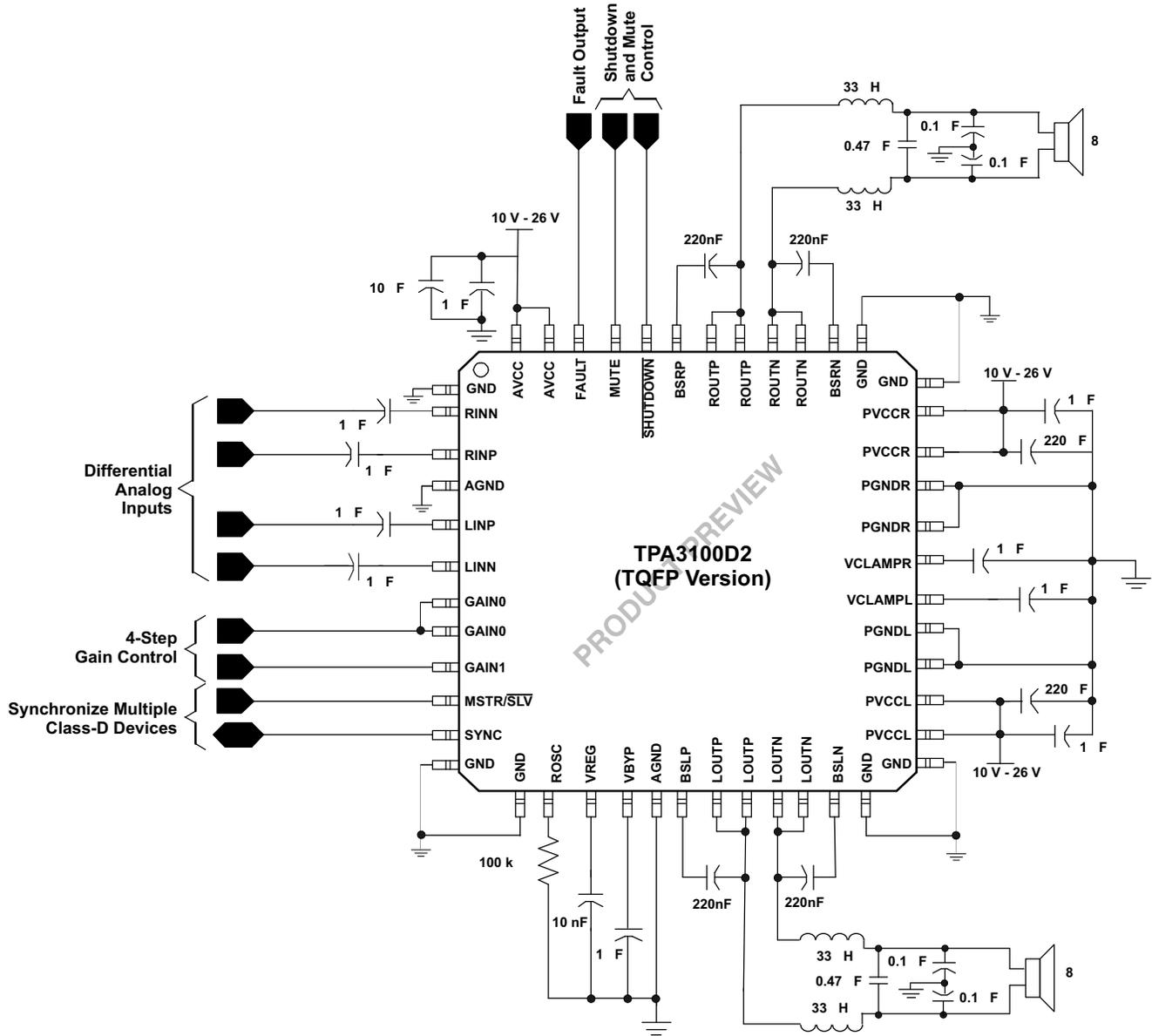
Figure 22. Stereo Class-D With Differential Inputs (TQFP)
