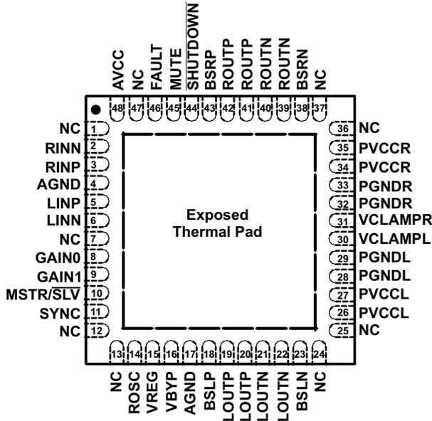
**48 PIN, TQFP PACKAGE
