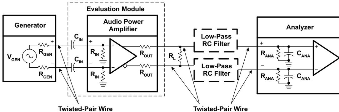
Figure 33. Differential Input, BTL Output Measurement Circuit
