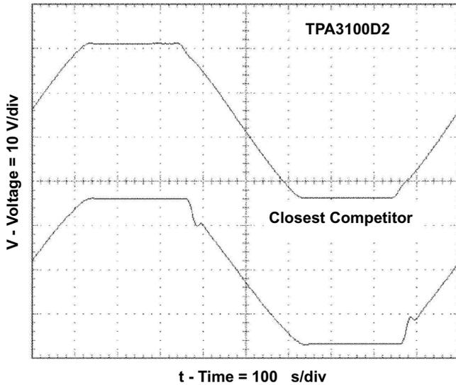
Figure 29. 1-kHz Sine Output at 10% THD+N
