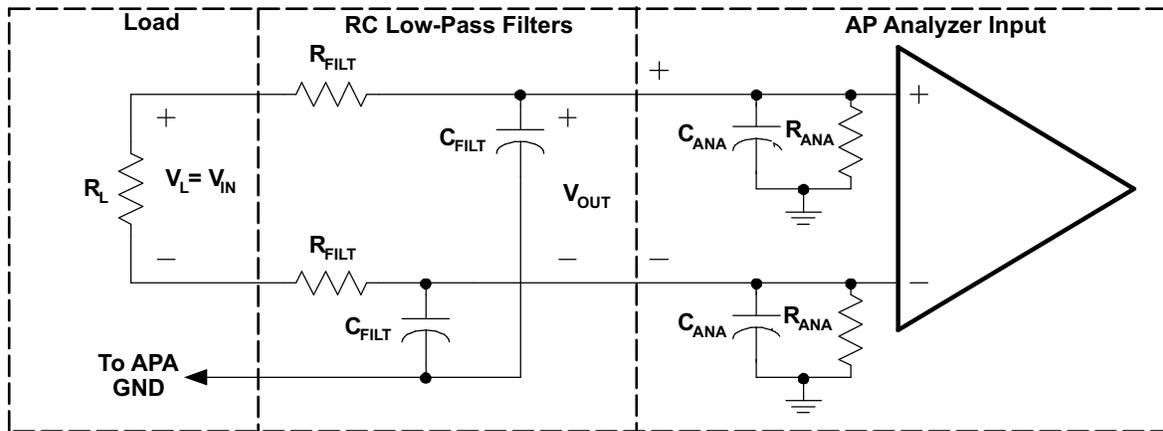
Figure 34. Measurement Low-Pass Filter Derivation Circuit-Class-D APAs
