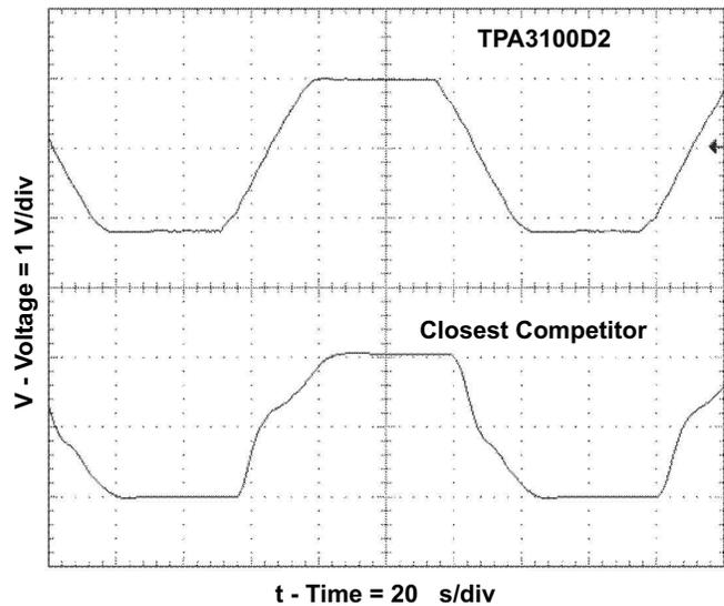
Figure 30. 8-kHz Sine Output at 10% THD+N
