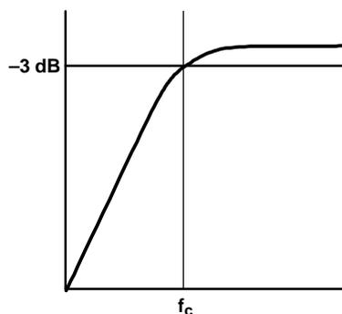
The value of  $C_{\text{I}}$  is important to consider as it directly affects the bass (low frequency) performance of the circuit. Consider the example where  $R_{\text{I}}$  is 10 k $\Omega$  and the specification calls for a flat bass response down to 100 Hz. Equation 2 is reconfigured as Equation 3.
