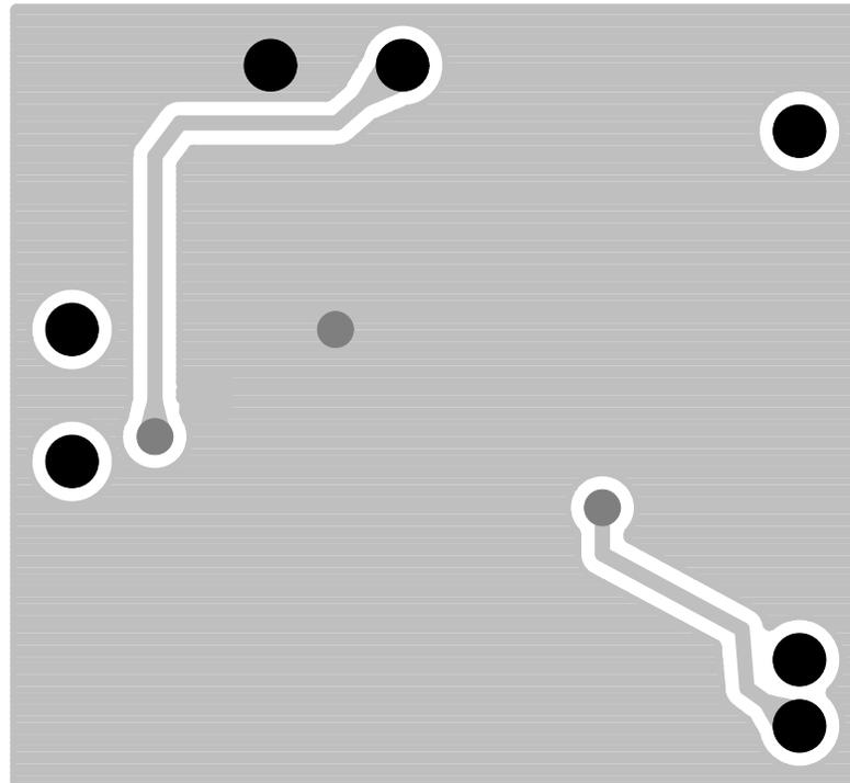
Figure 36. TPA6203A1 EVM Bottom Layer (Not to scale)
