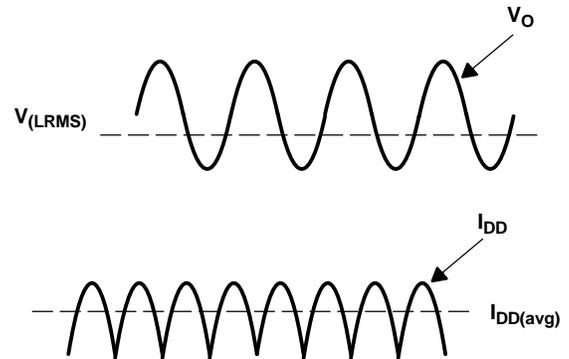
**Figure 33. Voltage and Current Waveforms for BTL Amplifiers**
