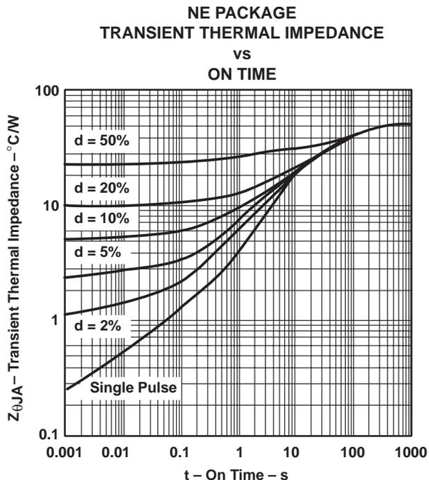
The single-pulse curve represents measured data. The curves for various pulse durations are based on the following equation:
