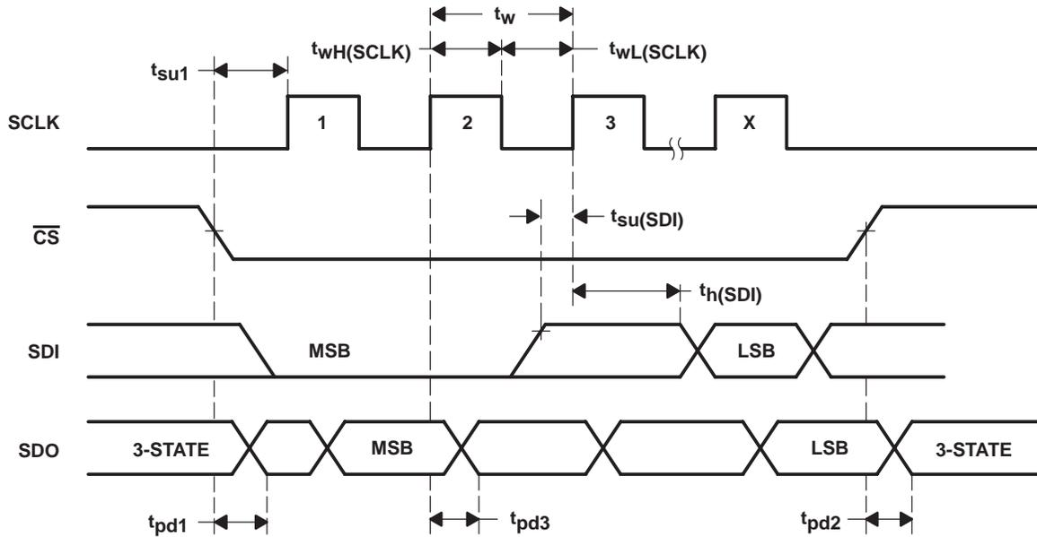
Figure 1. Switching Characteristics
