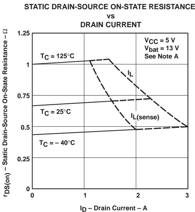
NOTE A: Technique should limit  $T_J - T_C$  to 10°C maximum.
