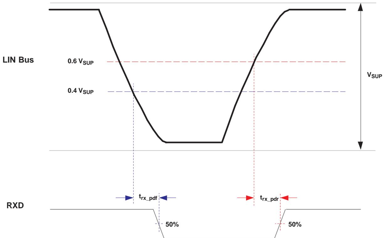
Figure 6. Propagation Delay
