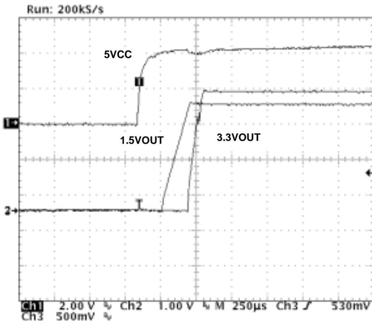
NOTE: The outputs track within 2 V in the power-up and power-down sequence.
