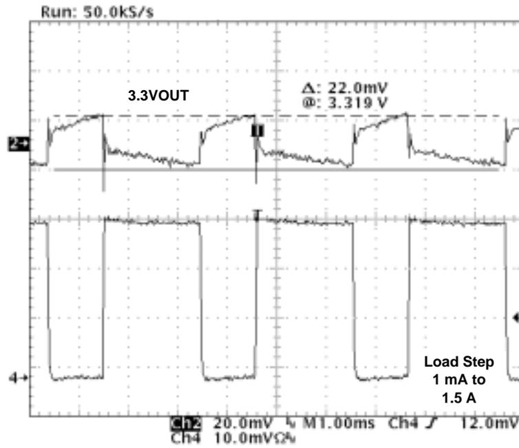
NOTE: Load regulation on 3.3VOUT with a load step of 1 mA to 1.5 A
