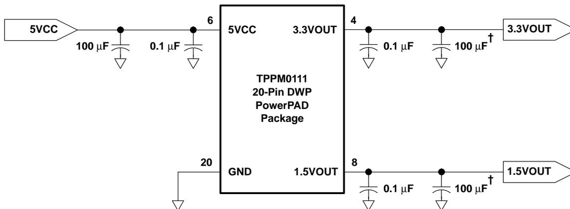
† It is recommended that the capacitors on the outputs (100 µF) have a low ESR < 1 Ω. These stabilizing capacitors must be placed in close proximity of their corresponding output terminals for optimal performance.
