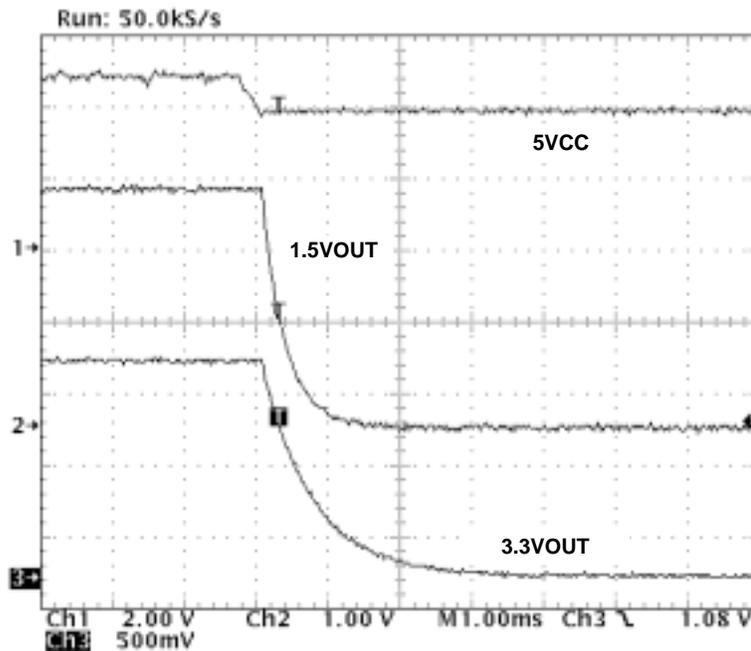
NOTE: The output tracks within 2 V in the power-down sequence.
