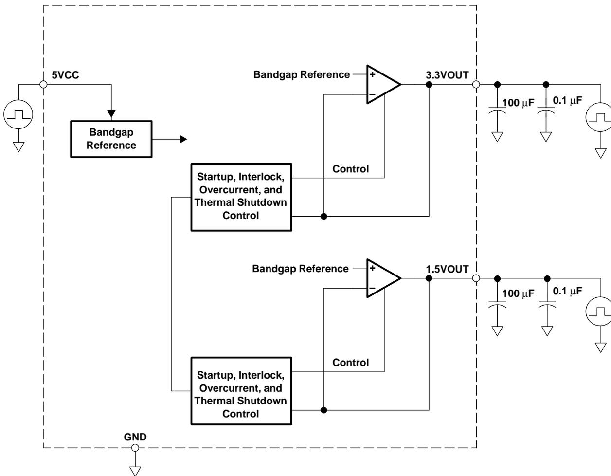
NOTE: The 100- $\mu\text{F}$  capacitor has: ESL = 3 nH and ESR = 0.5  $\Omega$  to 1  $\Omega$ .
