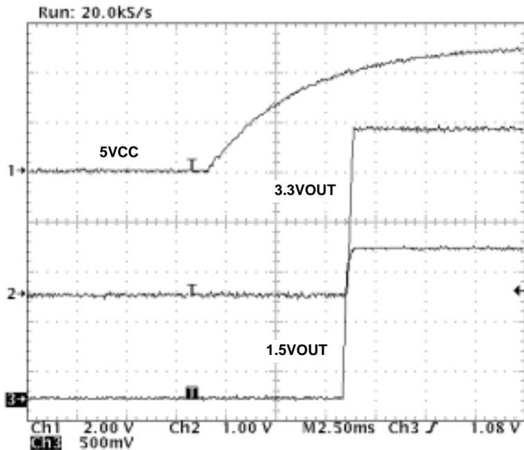
NOTE: The outputs track within 2 V in the power-up sequence.
