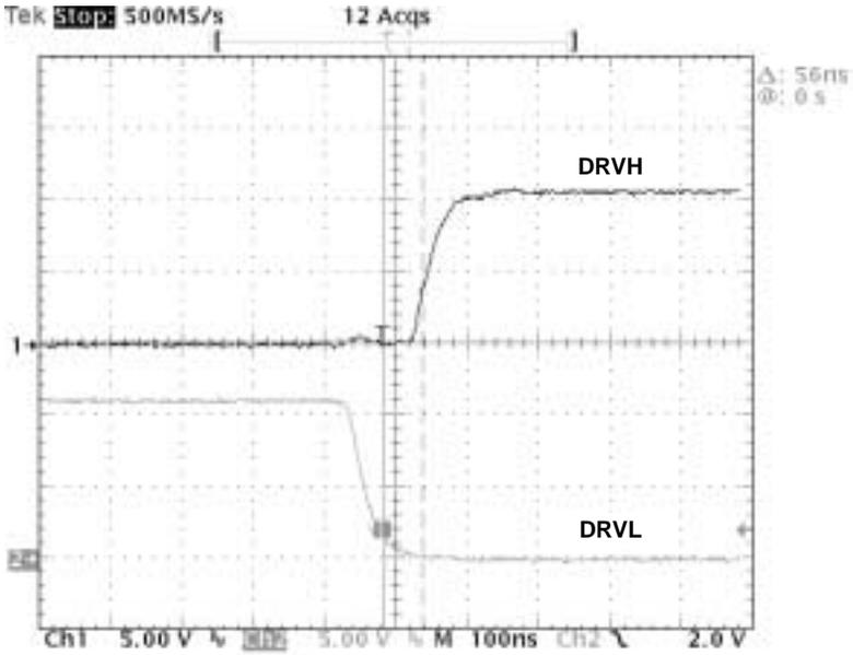
Figure 2. Dead Time Between Gate Drives Upper Switching ON and Lower Switching OFF
