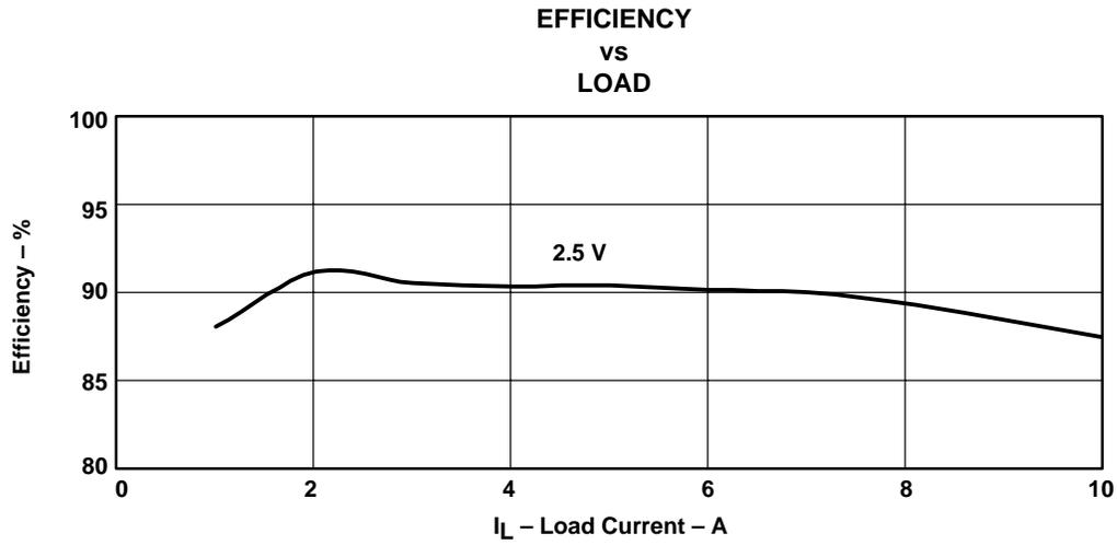
Figure 7. System Efficiency With Load Current (2.5-V Output)
