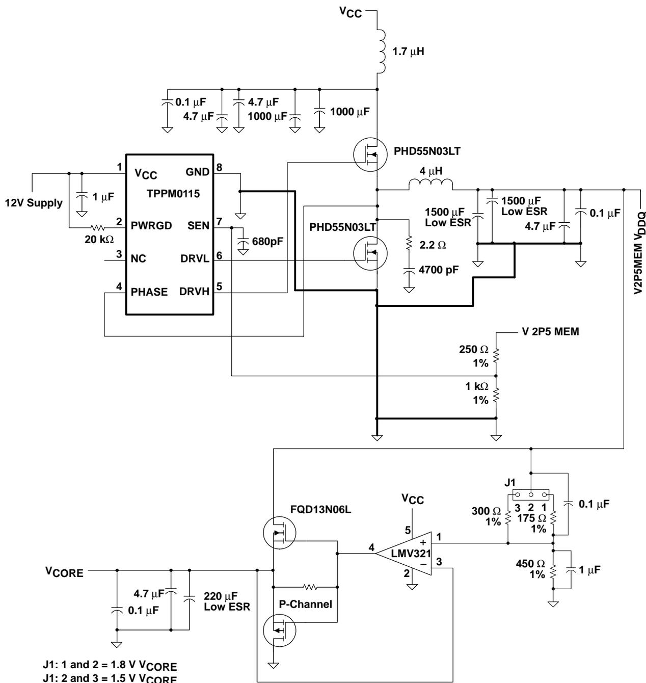
NOTES: A. The heavy lines must be kept short and connected to the ground plane construction for efficient results.
