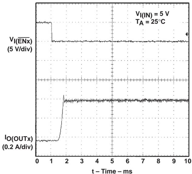
Figure 6. TPS2046, Short-Circuit Current, Device Enabled into Short
