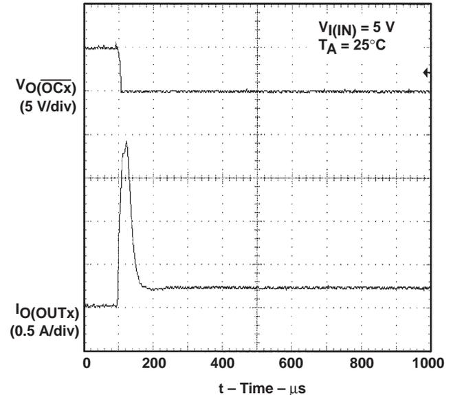
Figure 11. 1- $\Omega$  Load Connected to Enabled Device
