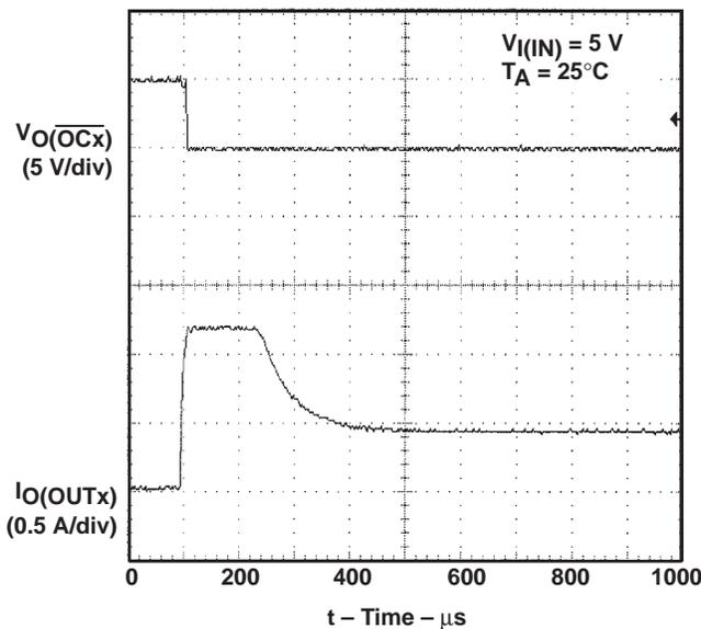
Figure 10. 4- $\Omega$  Load Connected to Enabled Device
