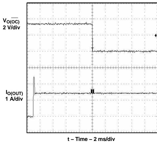
Figure 8. 2- $\Omega$  Load Connected to Enabled Device
