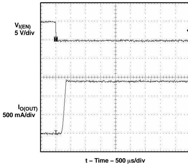
Figure 6. Short-Circuit Current, Device Enabled Into Short
