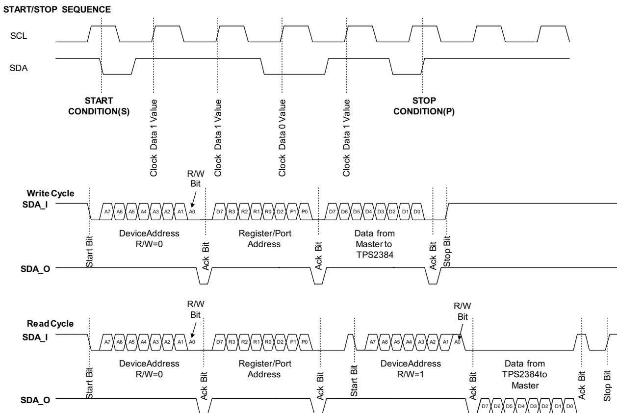
**Figure 16. I<sup>2</sup>C Read/Write Cycles**
