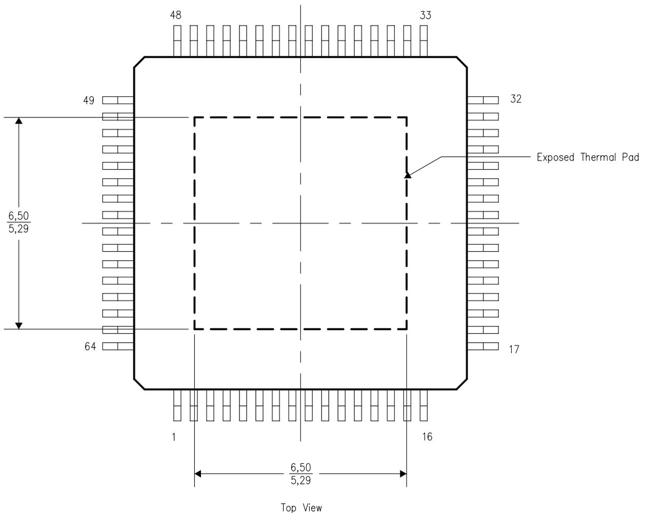
NOTE: All linear dimensions are in millimeters
