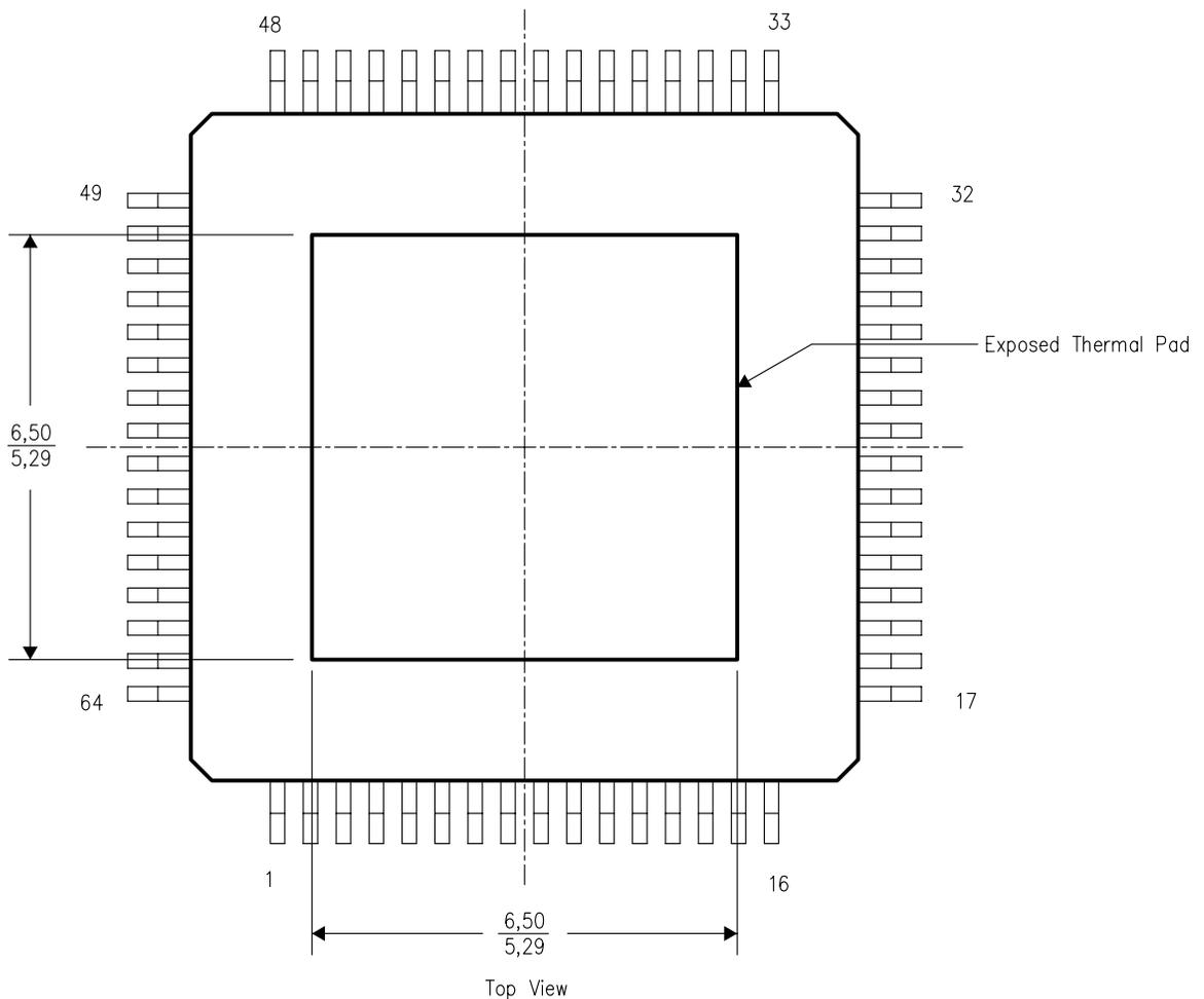
NOTE: All linear dimensions are in millimeters
