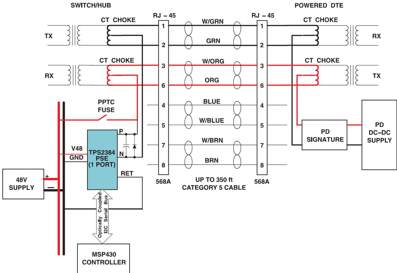
NOTE: A fuse may be required to provide additional protection if isolation is lost or the low-side current sense fails.
