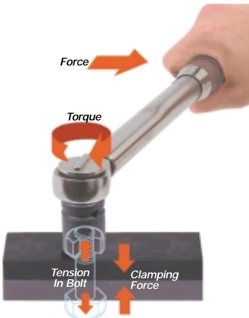
When torque is applied to the head of a bolt during a fastening process, there are actually two main forces at work. First, we are applying a force - torque to the bolt head to tighten it. The second force at work is the tension or stretch created that runs the length of the bolt.
