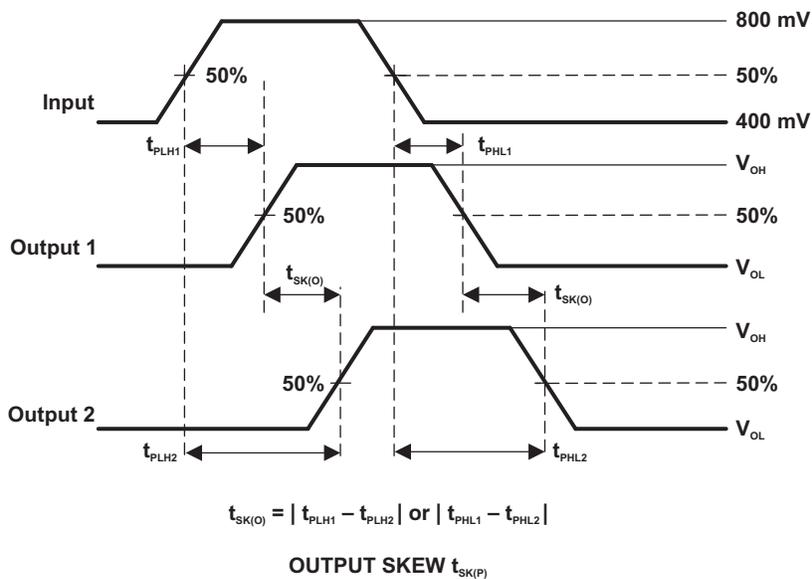
Figure 14. Skew Test
