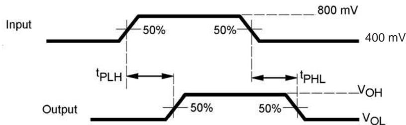
**Figure 13. Propagation Delay**
