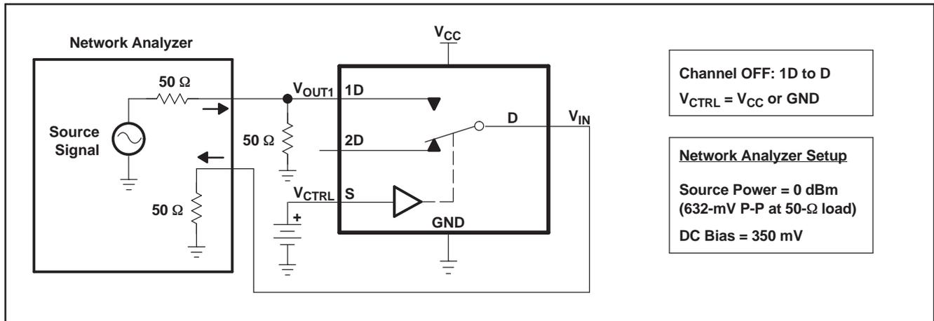
**Figure 10. OFF Isolation (O<sub>ISO</sub>)**
