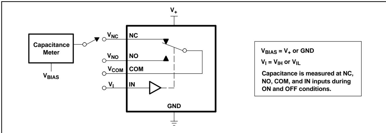
**Figure 16. Capacitance ( $C_I$ ,  $C_{COM(ON)}$ ,  $C_{NC(OFF)}$ ,  $C_{NO(OFF)}$ ,  $C_{NC(ON)}$ ,  $C_{NO(ON)}$ )**
