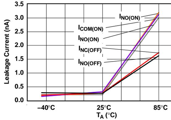
Figure 4. Leakage Current vs Temperature ( $V_+ = 5.5 \text{ V}$ )
