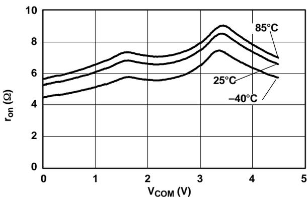
Figure 3.  $r_{on}$  vs  $V_{COM}$  ( $V_+ = 4.5\text{ V}$ )
