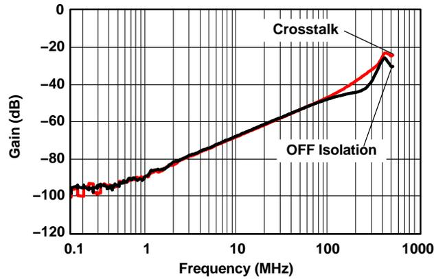
Figure 10. OFF Isolation ( $V_+ = 5\text{ V}$ )
