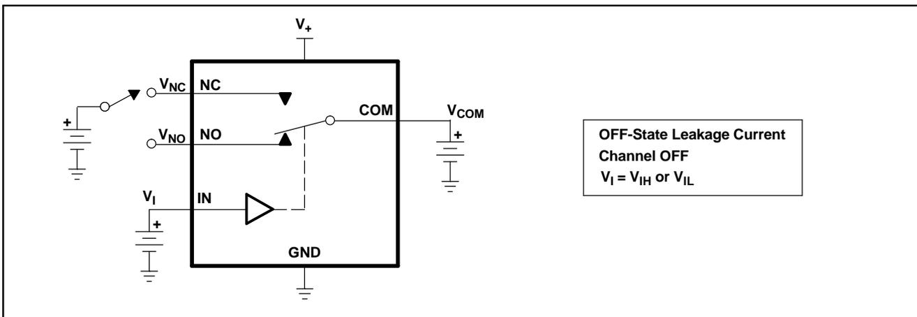
**Figure 14. OFF-State Leakage Current ( $I_{NC(OFF)}$ ,  $I_{NO(OFF)}$ )**
