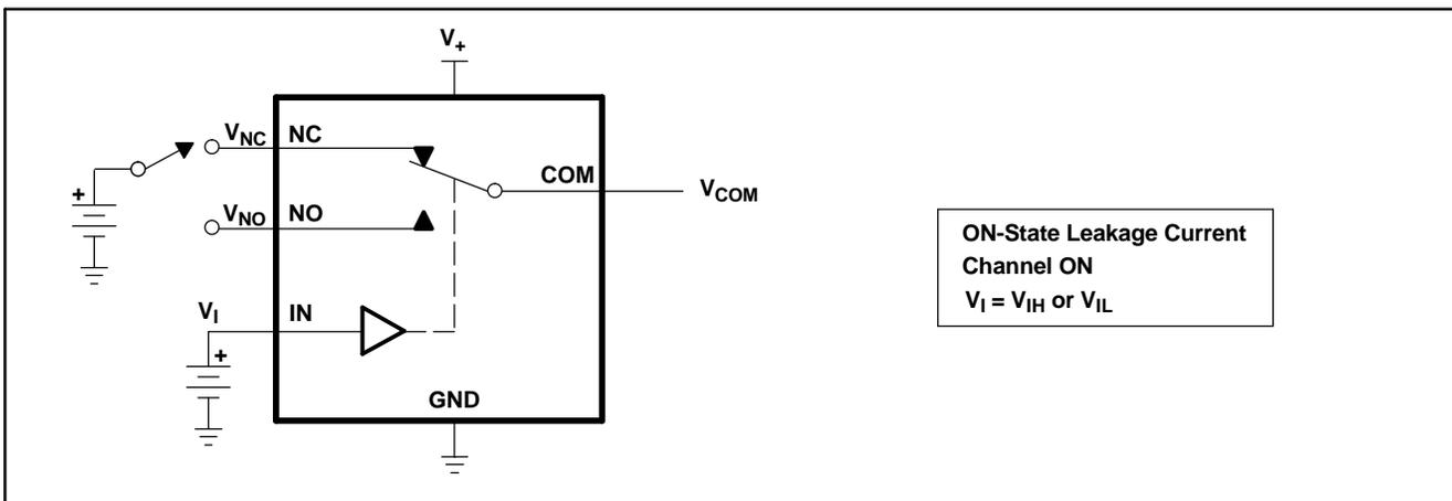
**Figure 15. ON-State Leakage Current ( $I_{COM(ON)}$ ,  $I_{NC(ON)}$ ,  $I_{NO(ON)}$ )**
