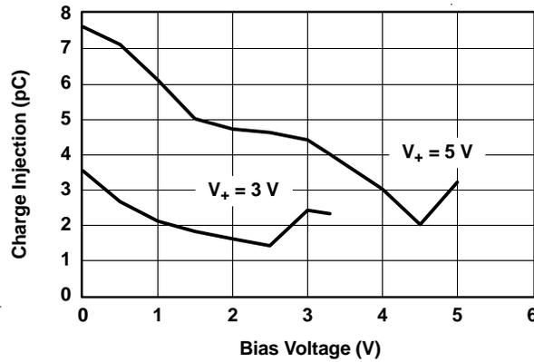
Figure 5. Charge Injection ( $Q_C$ ) vs  $V_{COM}$
