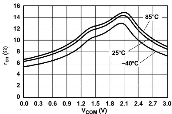
Figure 2.  $r_{on}$  vs  $V_{COM}$  ( $V_+ = 3\text{ V}$ )
