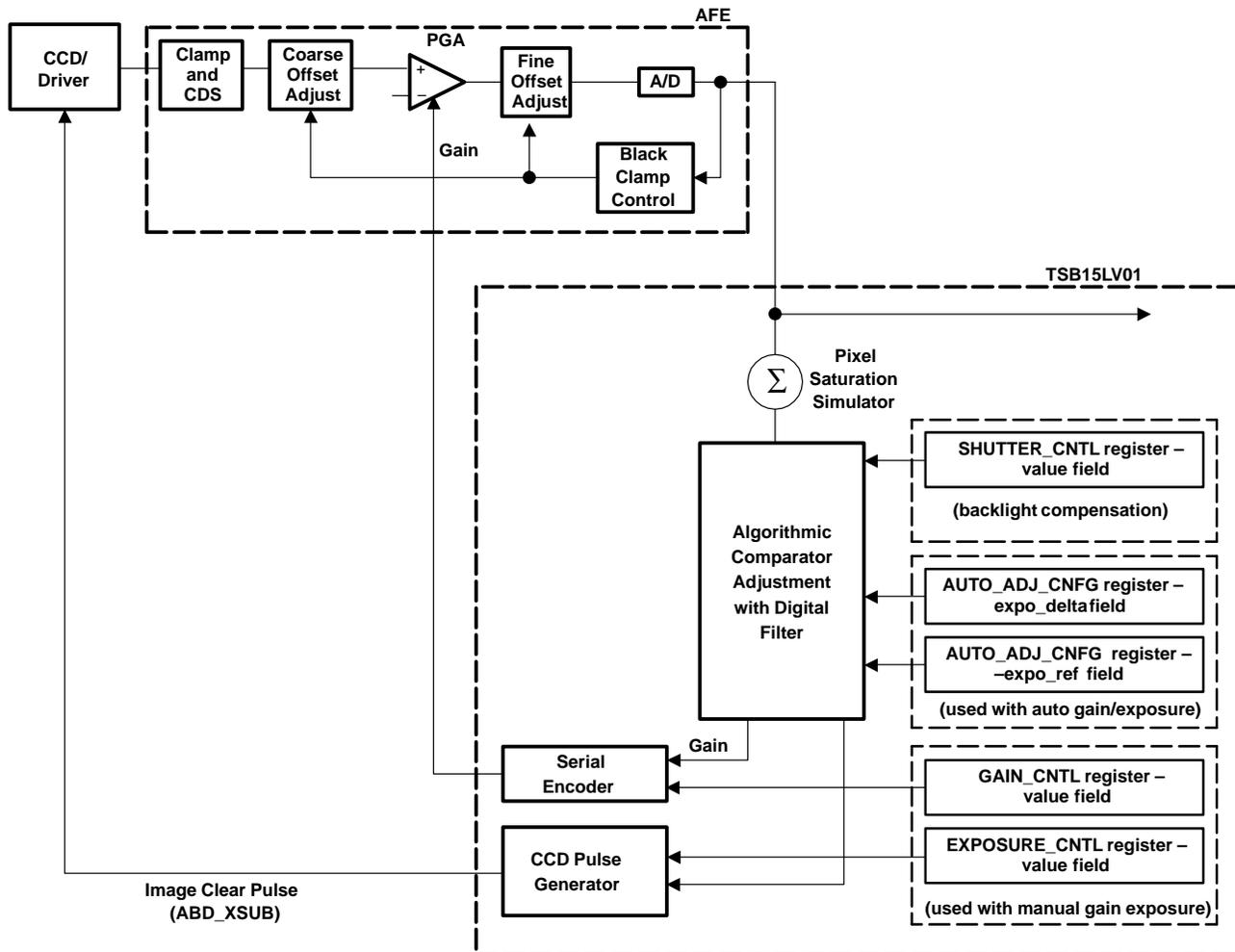
**Figure 2–16. Gain and Exposure Automatic and Manual Controls**
