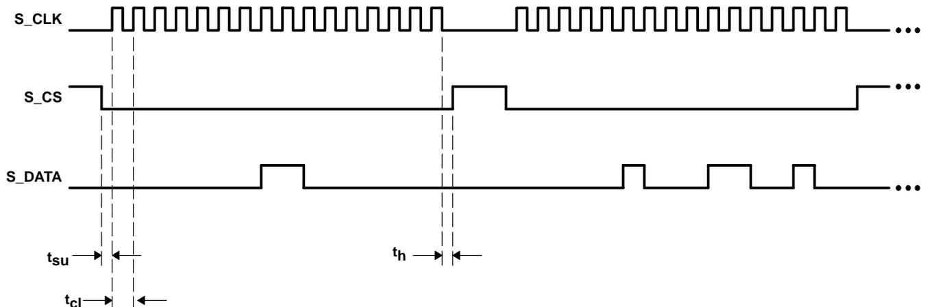
**Figure 2–3. AFE Serial Interface Timing**
