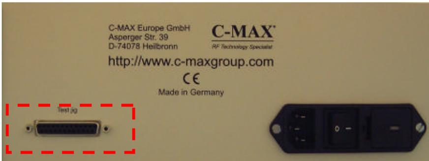
The test jig must be connected to the SUB25 parallel connector at the back side of the TSG800.
