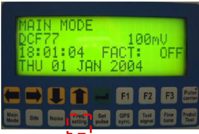
To activate the FREQUENCY ADJUST MODE, the button FREQ. SETTING must be pushed.
