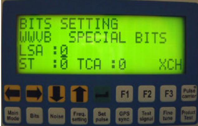
Furthermore, the announcement bit for the leap second can be switched (LSA L= Leap Second Announcement)
