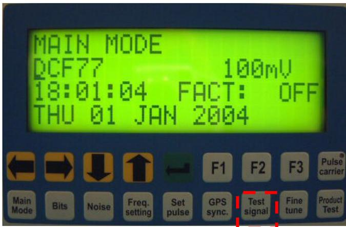
To activate the TEST SIGNAL MODE, the button TEST SIGNAL must be pushed.
