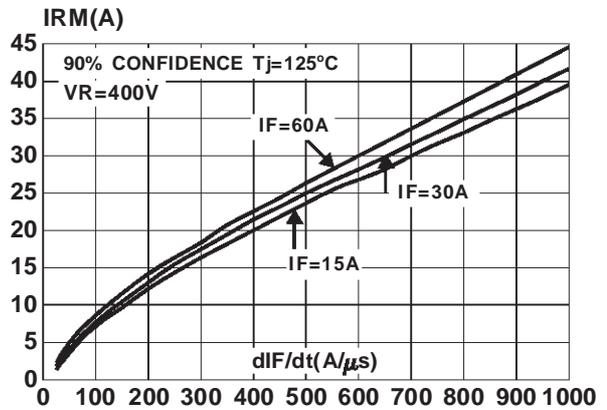
Fig. 5: Reverse recovery time versus  $dI_F/dt$ .
