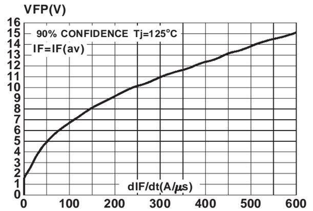
Fig. 9: Forward recovery time versus  $dI_F/dt$ .
