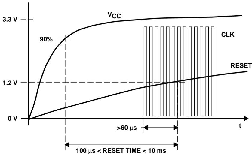
Figure 4–5. Reset Timing
