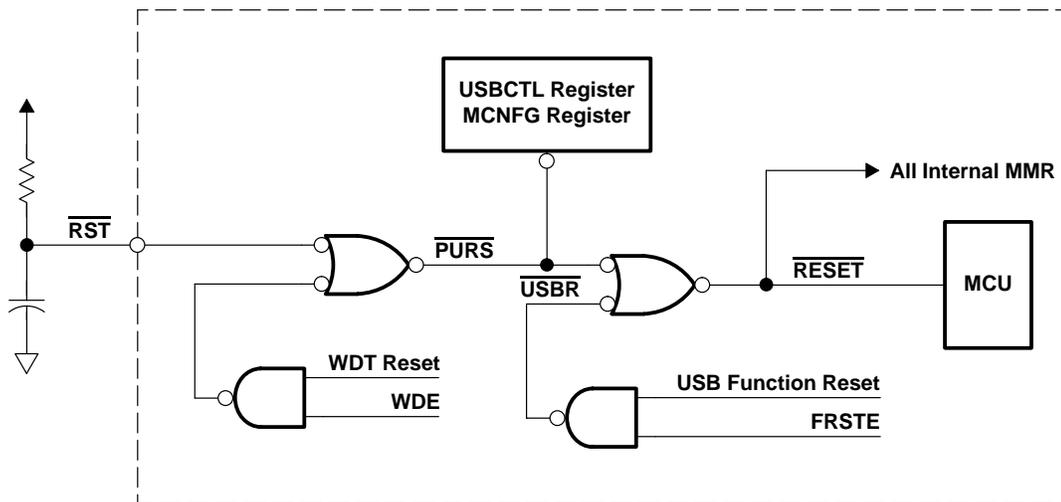
**Figure 2–3. Reset Diagram**
