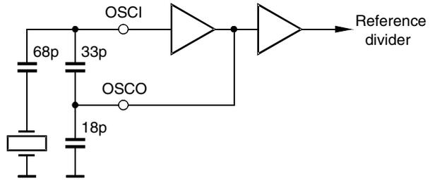
Figure 8. Oscillator Overdriven
