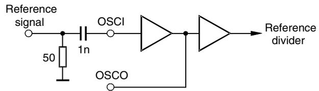
Figure 9. Measurement Circuit for Electrical Characteristics
