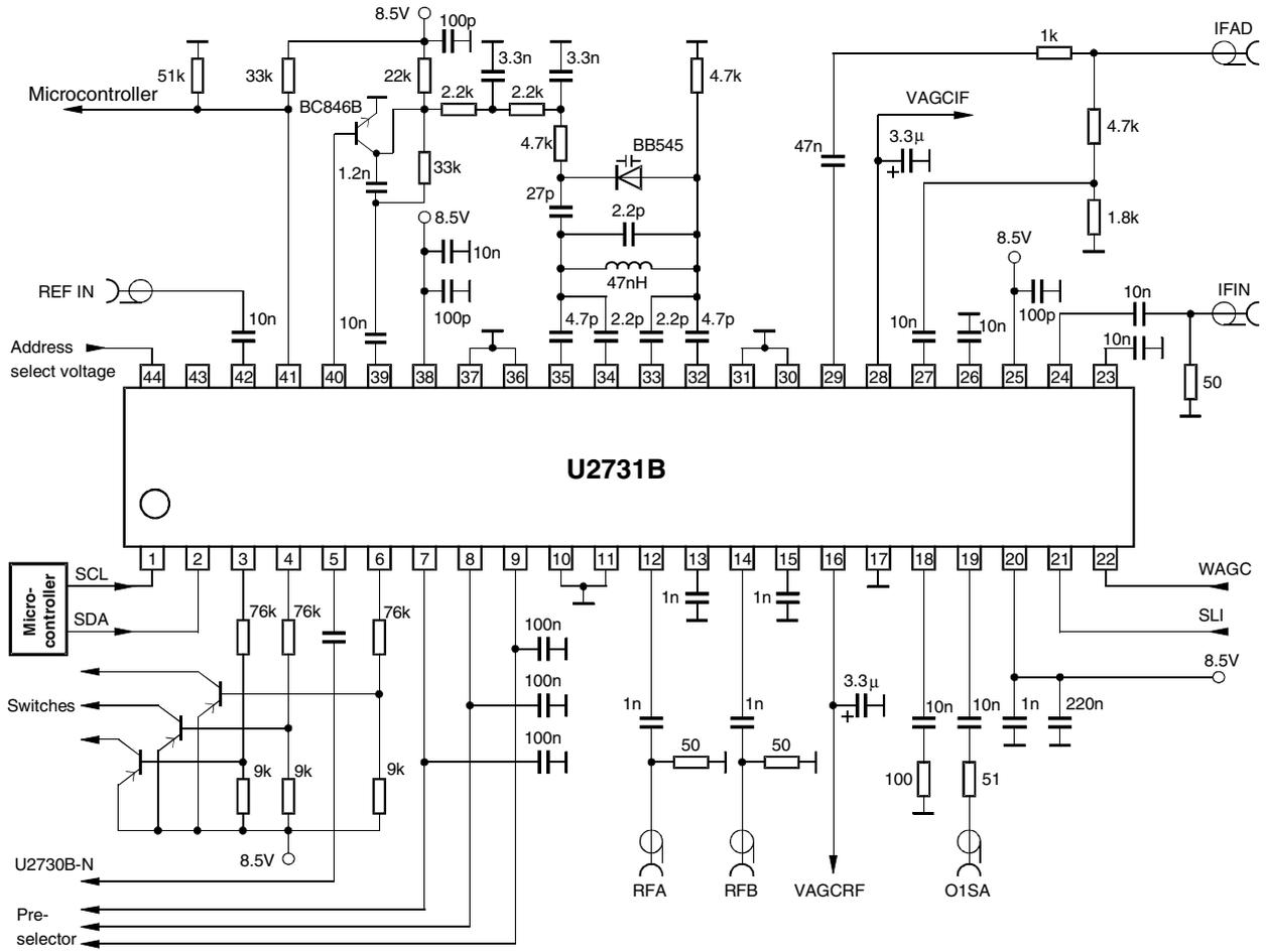
**Figure 10. RFAGC Voltage-generation Block Circuit**
