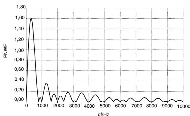
It is important to realize that this function shows zeros in all distances from the center line which are multiples of the carrier spacing. The technique of concentrating the phase noise in the positions of such zeros is patent protected.
