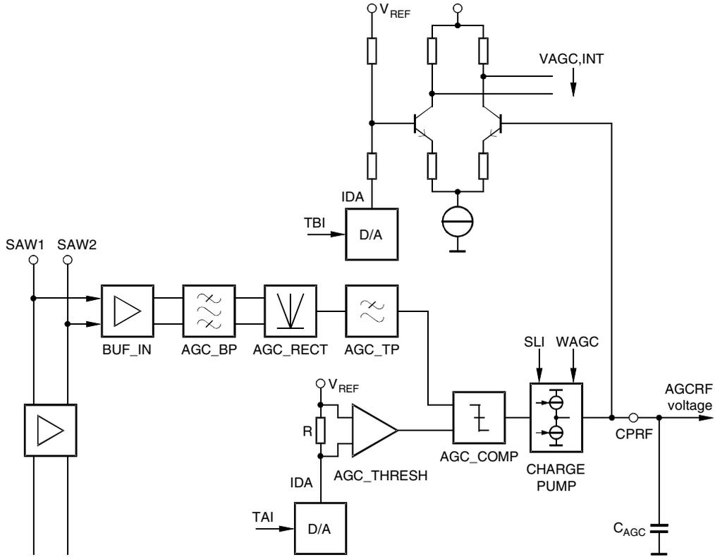
**Figure 11. IFAGC Voltage-generation Block Circuit**
