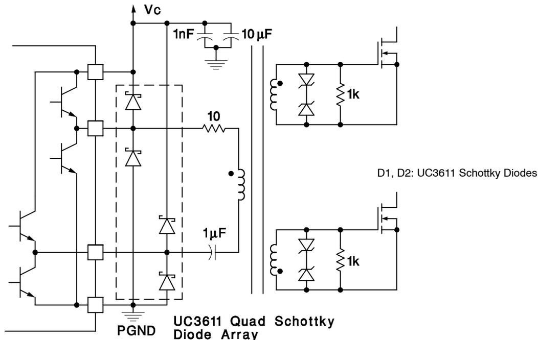
**Figure 4. Transformer coupled push-pull MOSFET drive circuit.**
