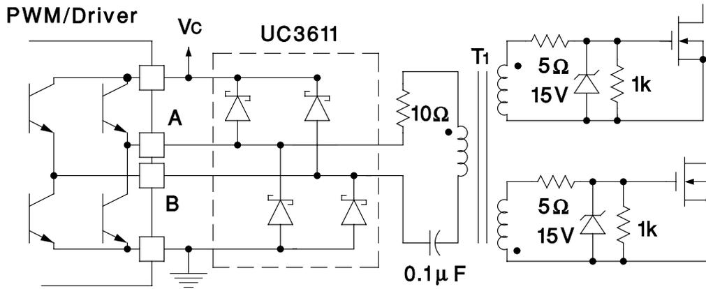
Figure 4. Transformer Coupled Drive Circuits
