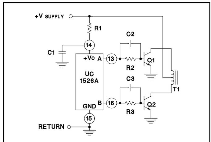
**Figure 7. Push-Pull Configuration**
