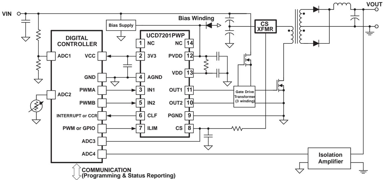
Figure 2. Half-Bridge Converter
