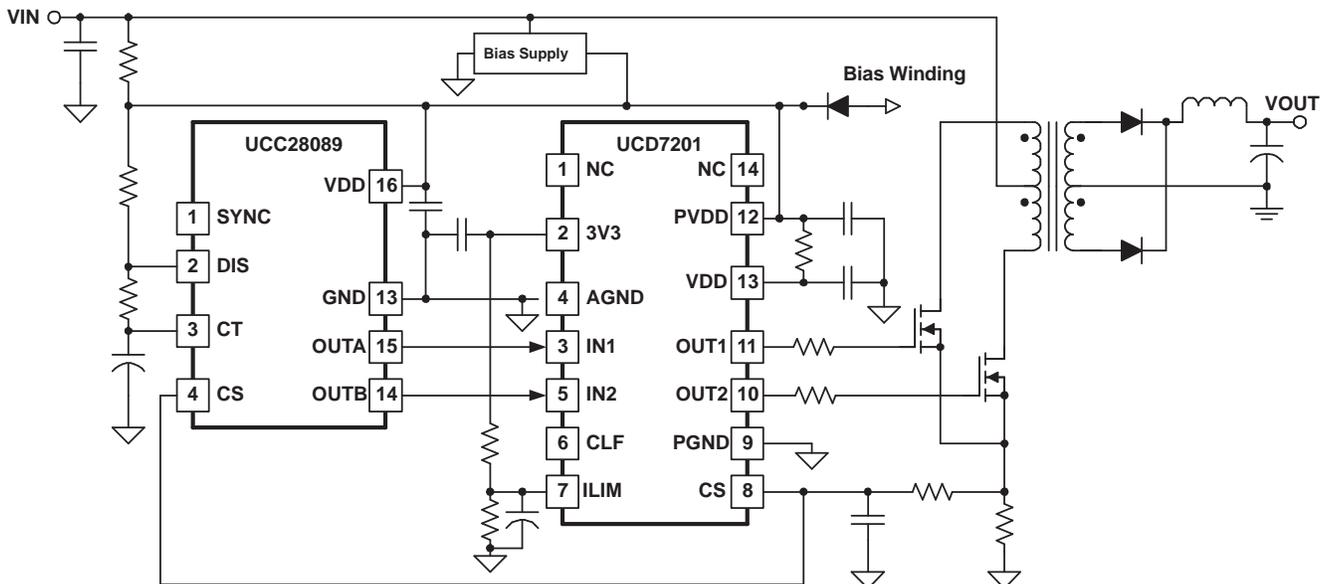
Figure 3. Intermediate Bus Converter
