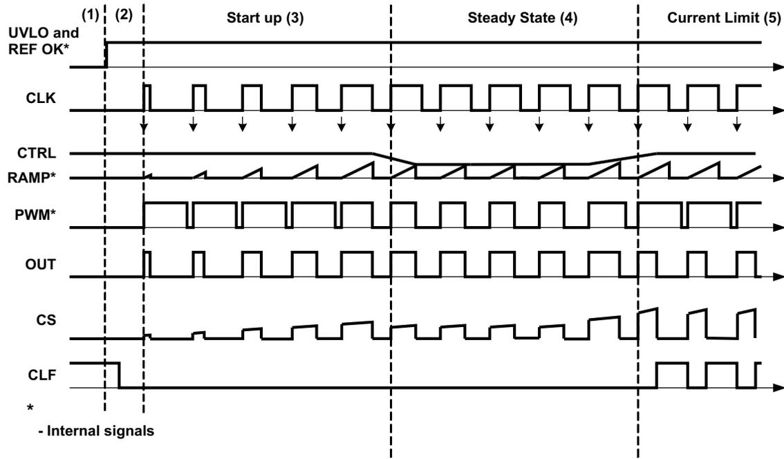
Figure 30. UCD8220 Timing and Circuit Operation Diagram
