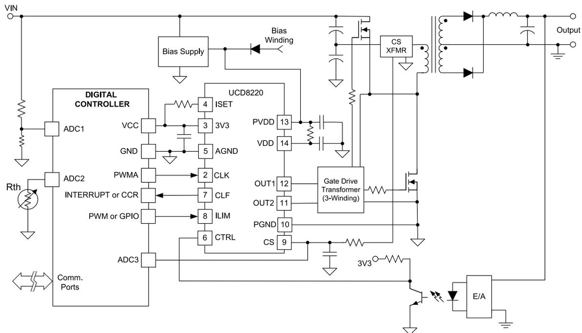
Figure 2. UCD8220 Typical Simplified Half-Bridge Converter Application Schematic
