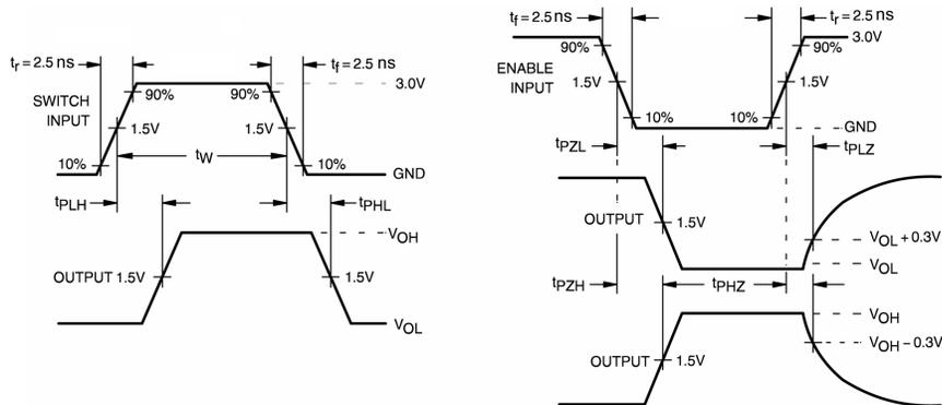
FIGURE 3. AC Waveforms
