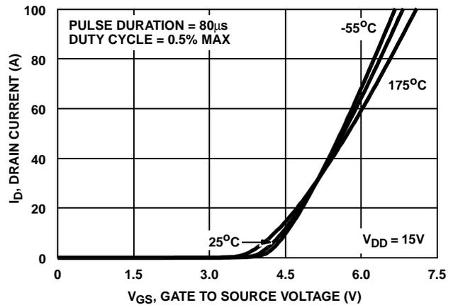
FIGURE 8. TRANSFER CHARACTERISTICS
