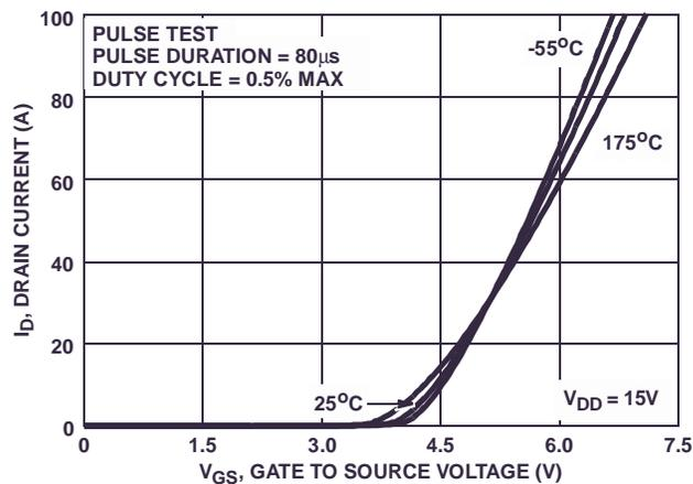
FIGURE 8. TRANSFER CHARACTERISTICS
