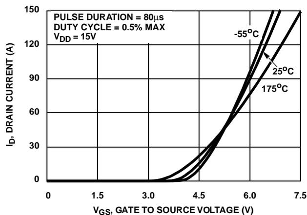
FIGURE 8. TRANSFER CHARACTERISTICS
