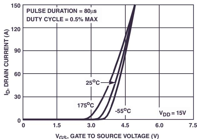
FIGURE 8. TRANSFER CHARACTERISTICS
