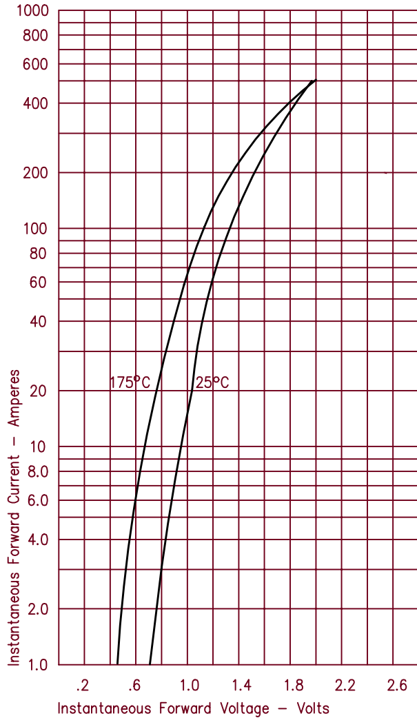
Figure 1 Typical Forward Characteristics – Per Leg
