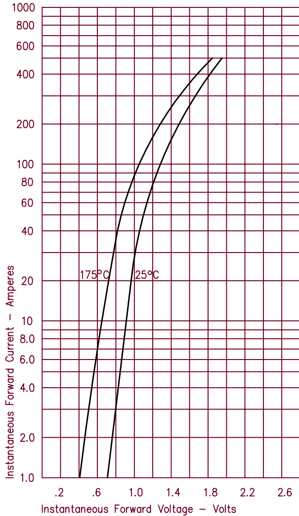
Figure 1 Typical Forward Characteristics – Per Leg
