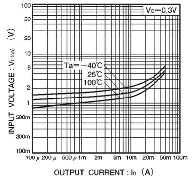
Fig.1 Input voltage vs. output current (ON characteristics)
