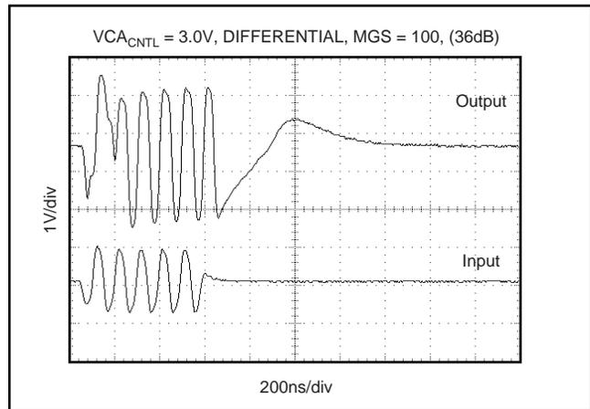
FIGURE 16. Overload Recovery Response For Maximum Gain.
