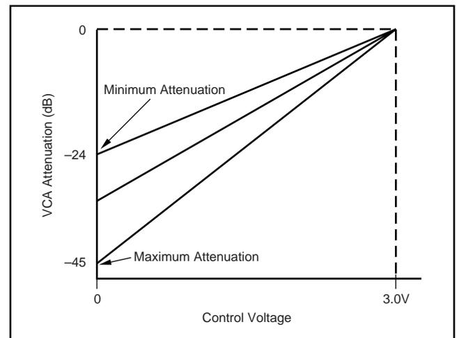
FIGURE 3. Swept Attenuator Characteristic.
