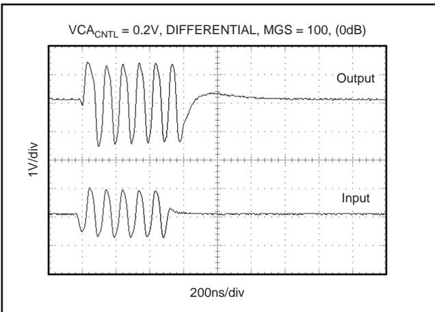
FIGURE 15. Overload Recovery Response For Minimum Gain.
