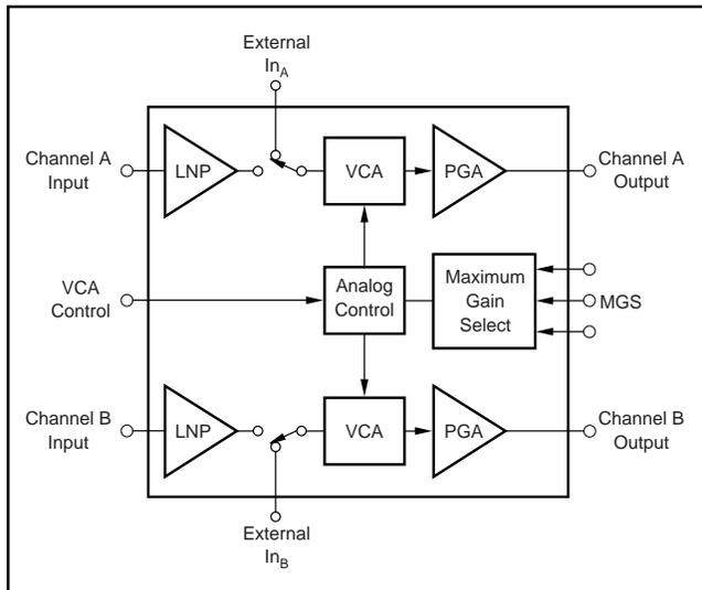
FIGURE 1. Simplified Block Diagram of the VCA2613.
