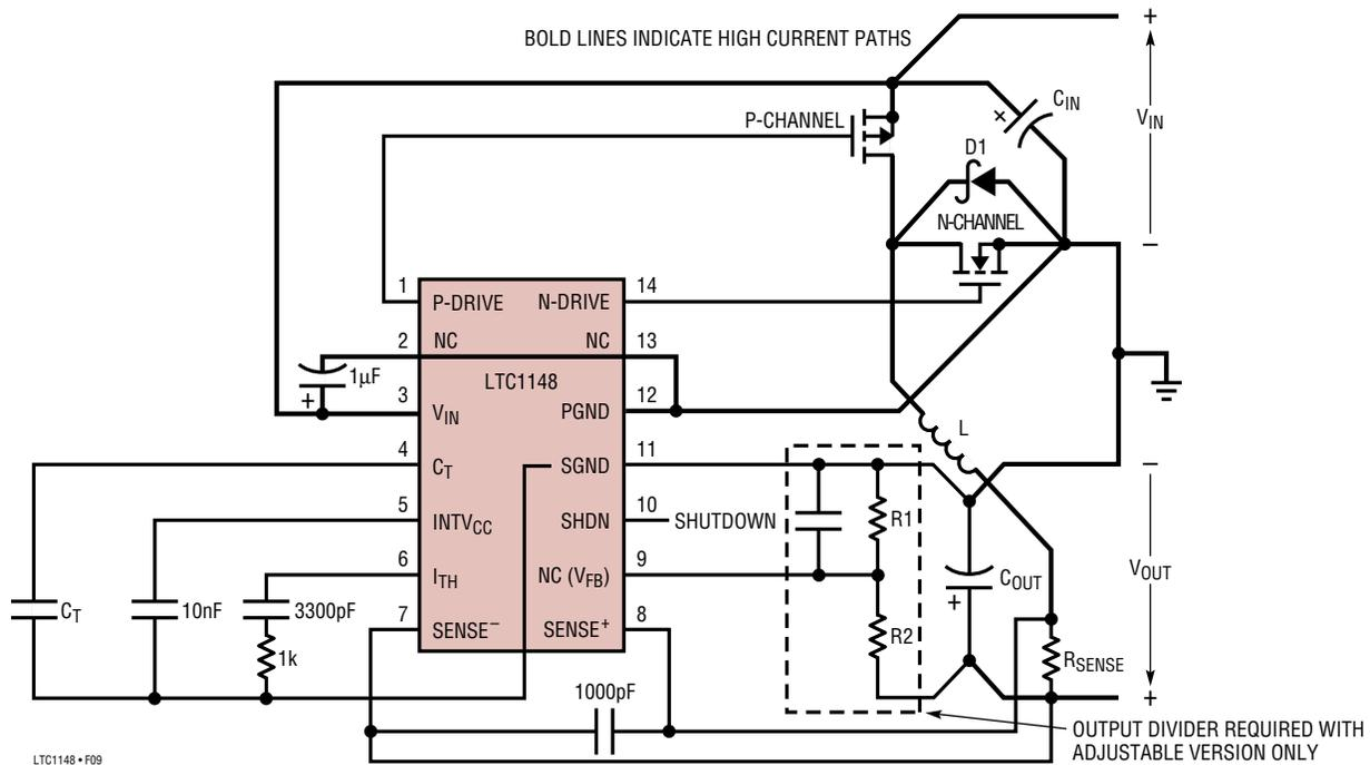
Figure 9. LTC1148 Layout Diagram (See Board Layout Checklist)
