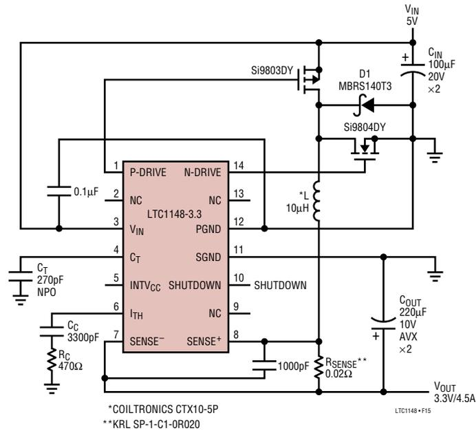
Figure 15. High Efficiency 5V to 3.3V/4.5A Converter
