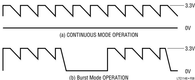
Figure 8.  $C_T$  Waveforms
