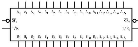
74VCX16245 Low Voltage 16-Bit Bidirectional Transceiver with 3.6V Tolerant Inputs and Outputs
