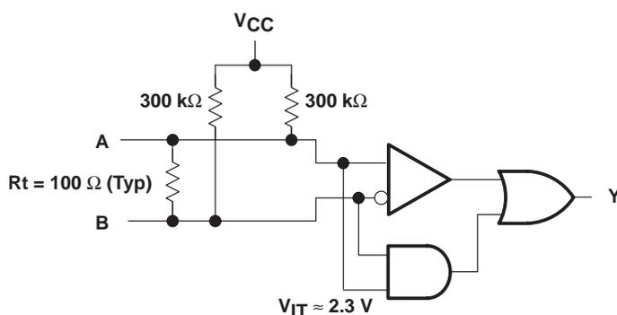
Figure 8. Open-Circuit Fail Safe of the LVDS Receiver
