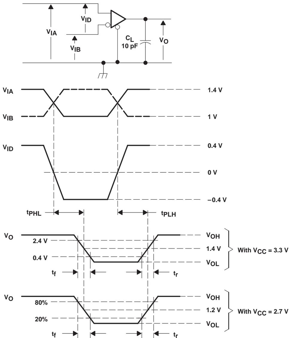
NOTE A: All input pulses are supplied by a generator having the following characteristics:  $t_r$  or  $t_f \leq 1 \text{ ns}$ , pulse repetition rate (PRR) = 50 Mpps, pulse width =  $10 \pm 0.2 \text{ ns}$ .  $C_L$  includes instrumentation and fixture capacitance within 0,06 m of the D.U.T.
