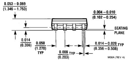
**8-Lead Small Outline Integrated Circuit (SOIC), JEDEC MS-012, 0.150" Narrow
