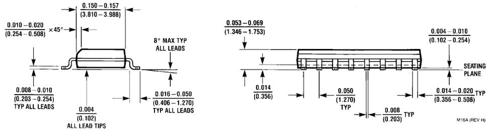
**16-Lead Small Outline Integrated Circuit (SOIC), JEDEC MS-012, 0.150 Narrow
