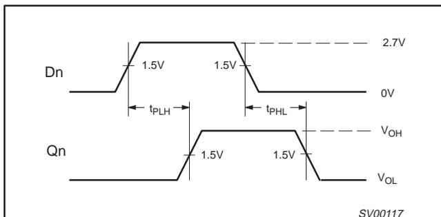
**Waveform 2. Propagation Delay for Data to Outputs**
