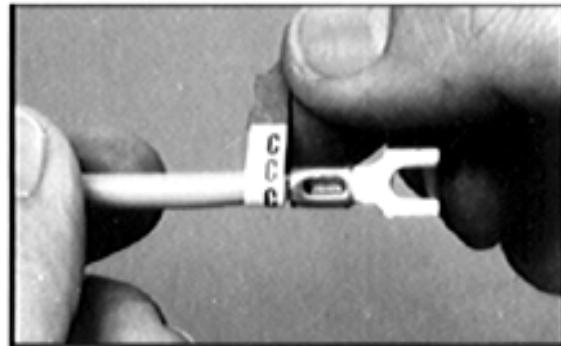
**Pick up tab to remove marker from book. Complete the wrap, and flip the tab off.**
