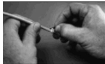
**Temporary Marking**-Wrap marker around wire. tab remains on. For permanent marking. flip off tab and press down.
