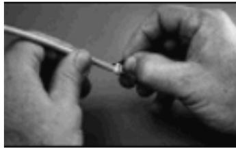
Temporary Marking-Wrap marker around wire. tab remains on. For permanent marking. flip off tab and press down.
