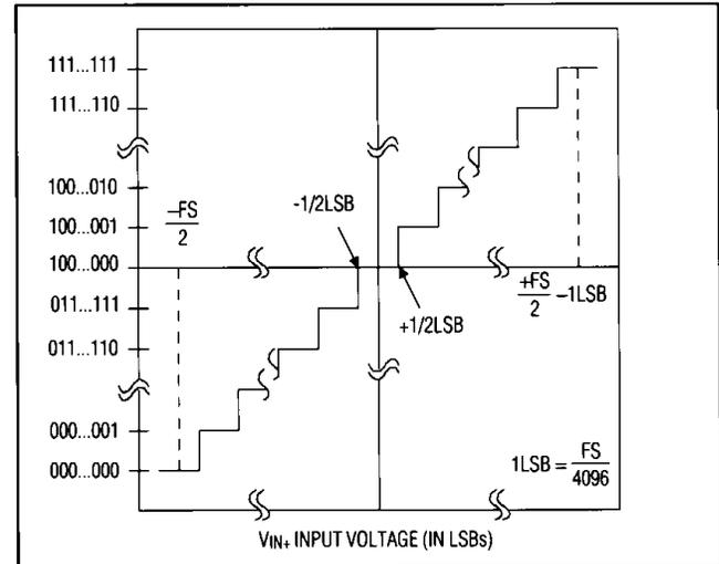
Figure 20. Ideal Input/Output Transfer Characteristic for Bipolar Operation
