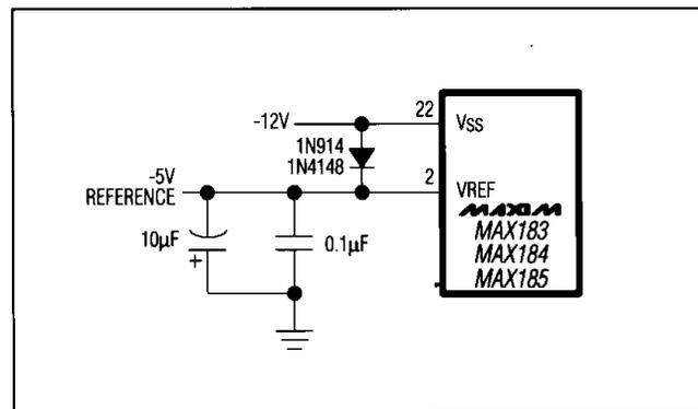
Figure 12. VREF/VSS Diode Clamp (See "Reference Input" Text).
