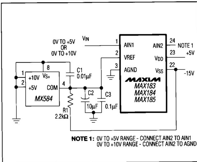
Figure 16. Unipolar Operation Using a MX584 Reference
