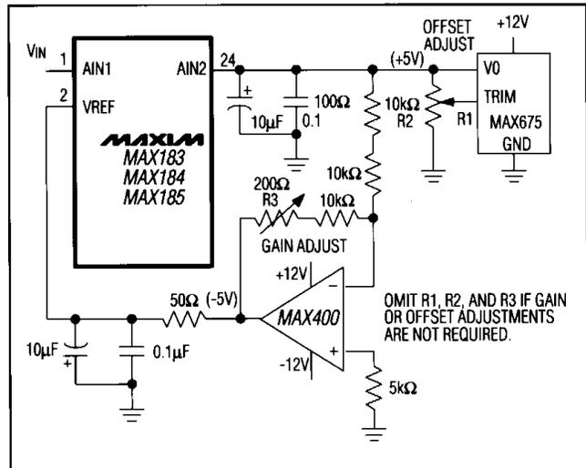
Figure 19. Bipolar Operation with Offset and Gain-Error Adjust
