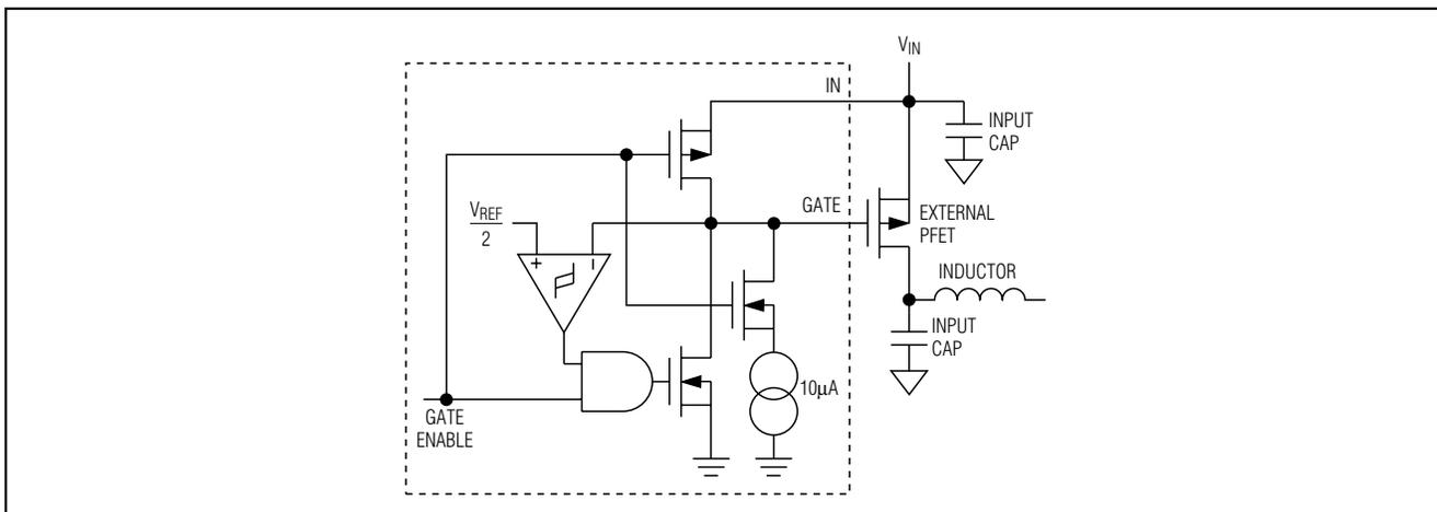
Figure 6. External P-Channel MOSFET Input Switch Control
