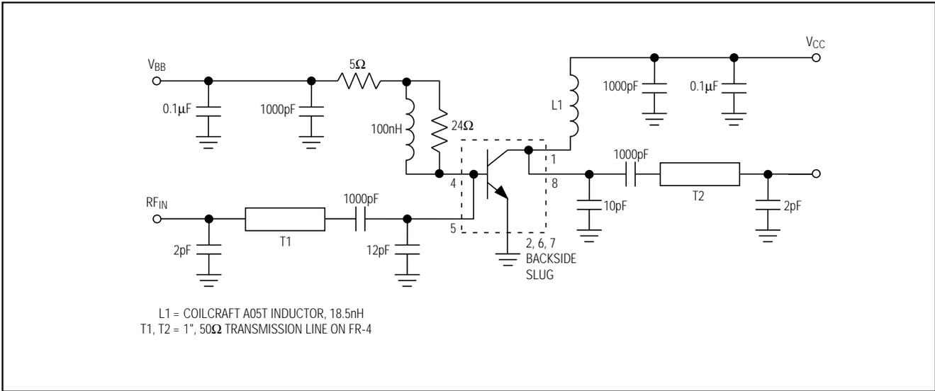
Figure 1. Test Circuit
