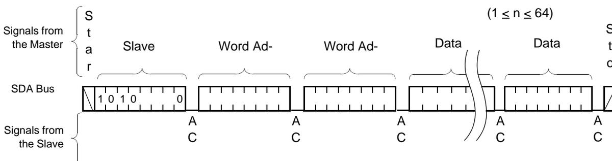
Figure 10. Writing 12 bytes to a 64-byte page starting at location 60.
