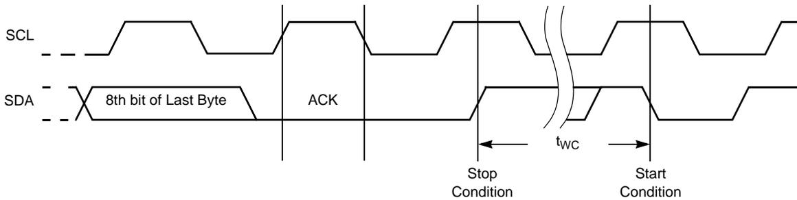
**Nonvolatile Write Cycle Timing**
