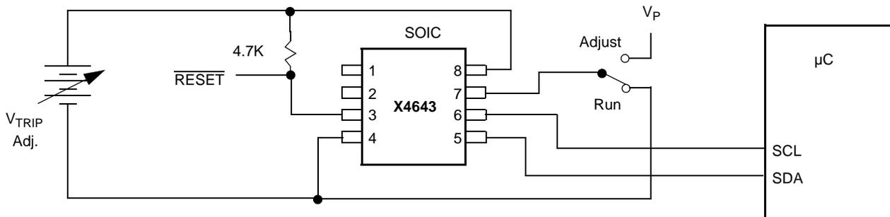
Figure 4.  $V_{TRIP}$  Programming Sequence
