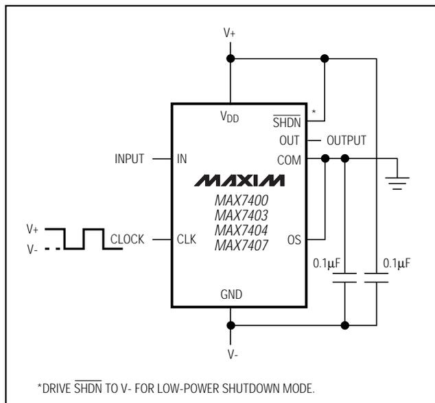
Figure 5. Dual-Supply Operation
