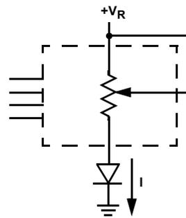
Two terminal Variable Resistor;
