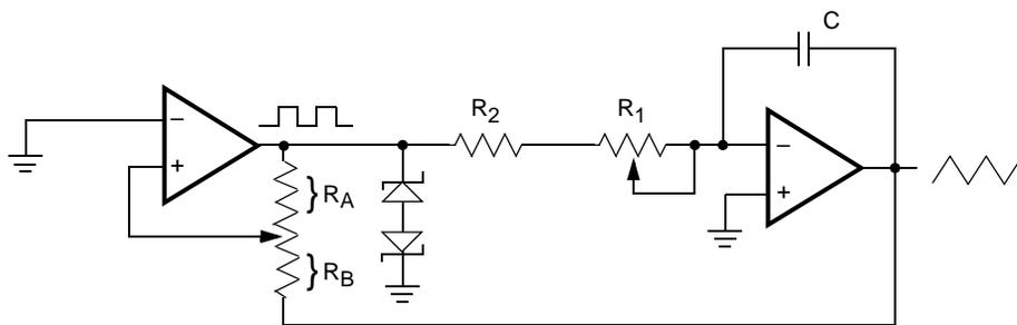
frequency  $\propto R_1, R_2, C$
