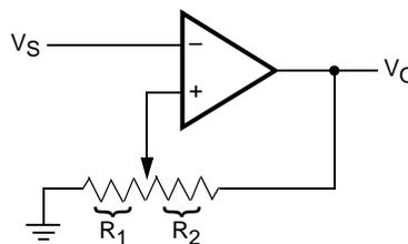
$$V_{UL} = \{R_1/(R_1 + R_2)\} V_O(\text{max})$$
